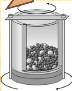
Mechanical Alloying (MA) by a planetary mill or an attritor device
